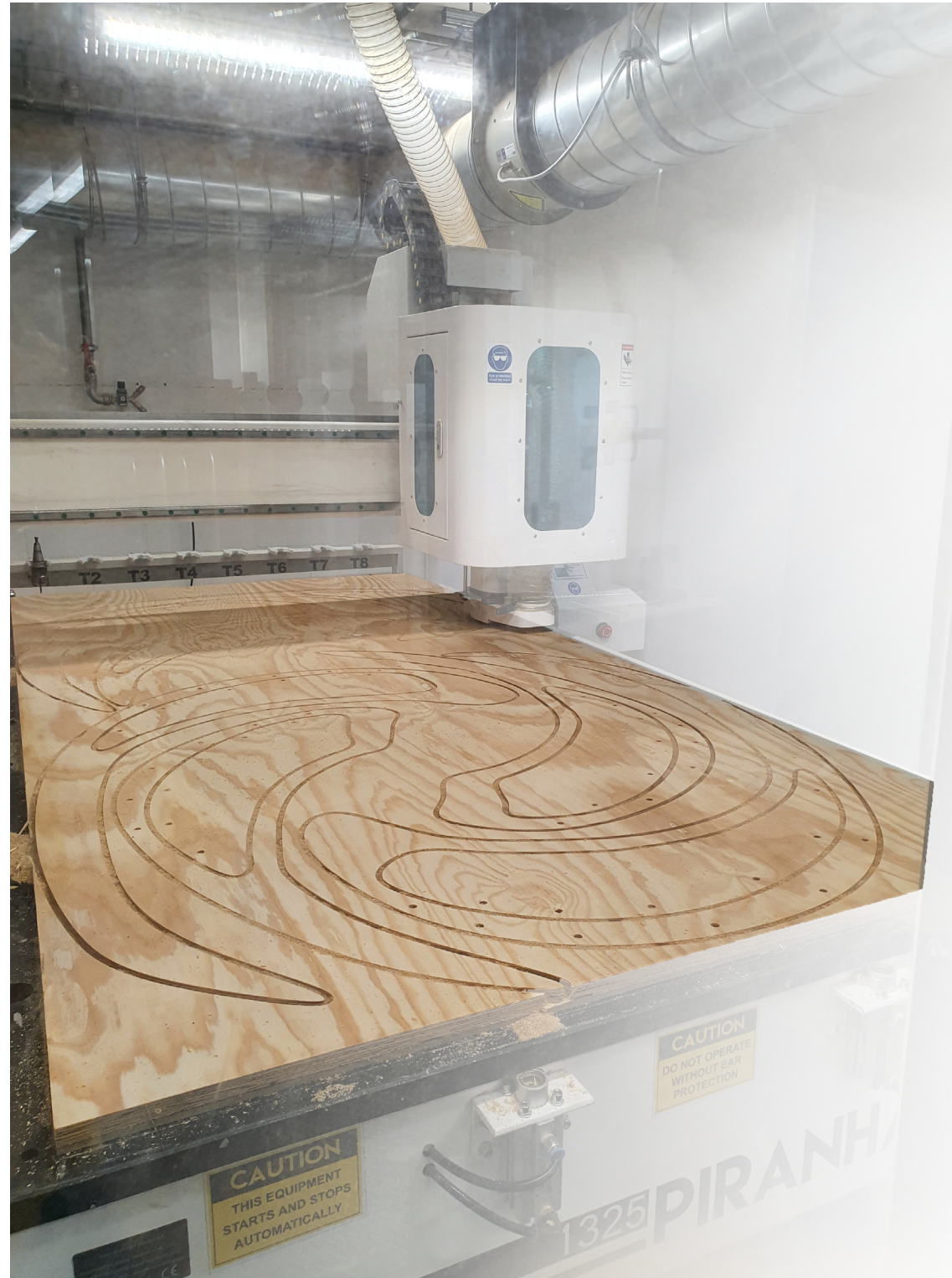
3. CNC cuts out 2D shape.
