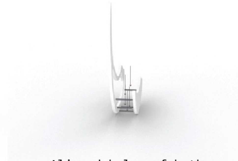
Aligned holes of both offcut and frame and insert rods
